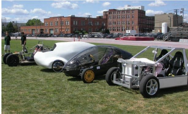
FINAL ALTERNATIVE-FUEL VEHICLES DESIGNED AND BUILT IN NINE WEEKS BY THE FOUR TEAMS PARTICIPATING IN THE VEHICLE DESIGN SUMMIT AT MIT, SUMMER 2006. FROM LEFT, THE FOUR DESIGNS ARE: BIOFUEL, ASSISTED HUMAN POWER VEHICLE, PULSE ELECTRIC, AND HYDROGEN FUEL CELL. (IMAGE COURTESY MIT VDS 1.0)
