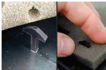
A DART CONNECTOR, WHICH REPLACES THE USE OF AN ADHESIVE, HOLDS ACOUSTIC FOAM SECURELY IN PLACE ON THE INSIDE OF A COMPUTER FRONT PANEL.
