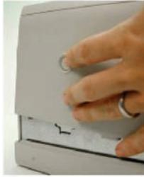
THIS DELL COMPUTER COVER IS OPENED BY SIMPLY PUSHING TWO BUTTONS ON EITHER SIDE OF THE COVER. NO TOOL IS REQUIRED AND THE CONNECTORS ARE INTEGRAL TO THEIR CORRESPONDING PARTS.
