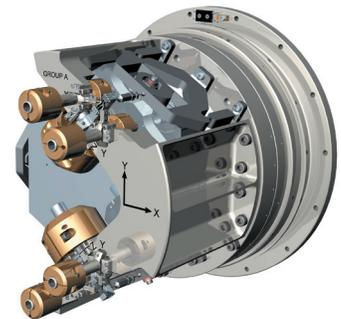
The optical bench (top) houses various optics, including lenses, mirrors, prisms, and gratings, as well as five rotary and three linear mechanisms. A mirror mount (bottom) uses counterweights to compensate for mirror tilt induced by gravity vector changes during observation.
